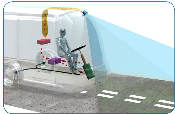
Image 2: Optiguide uses information from video cameras and other sensors to automatically steer the bus.
