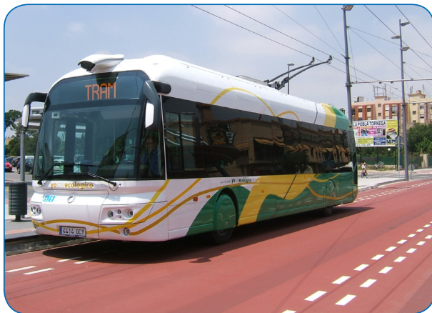
Image 1: By using road markings the Siemens Optiguide steers the bus automatically to within 5 cm of the bus stop.
