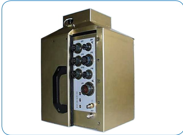
Image 3: The control computer is based on the Kontron PC/104-Plus SBC MICROSPACE® MSM800SEL and the framegrabber MICROSPACE® MSMG104.
