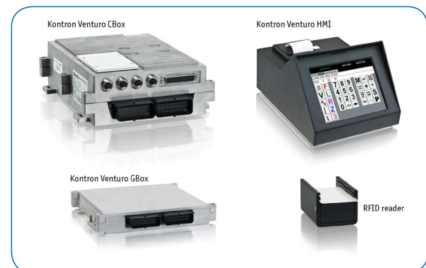
Image 2: The components of the vehicle management system from Kontron: The central computer is connected to the driver's console, GSM Voice & audio box and RFID reader.
